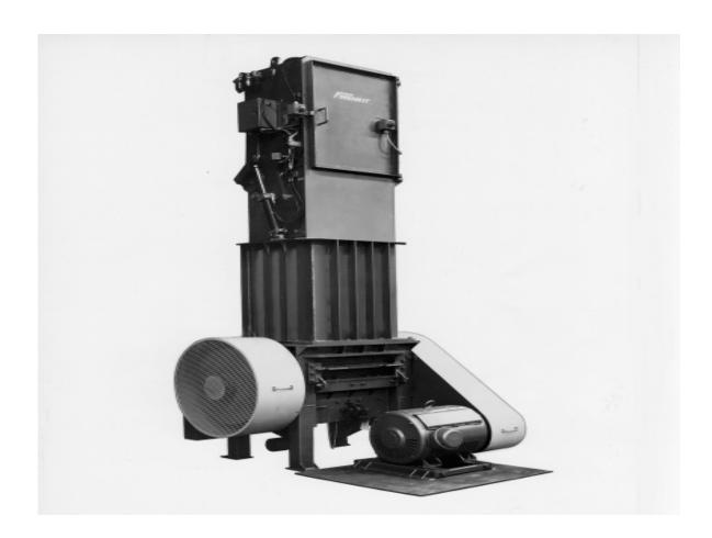
Foremost's new 30" X 30" large barrel grinder is intended for pit mounting and features an over 1000 lb flywheel, pneumatically operated feed control with direct vertical drop, and numerous servicing convenience features.
