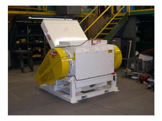
The SHD-9A **scrap grinders** are specifically designed and built to granulate either large parts or high volumes of scrap material. With its large throat size of 24" x 48", offset cutting chamber and rugged construction, large molded parts can be readily granulated without the need for pre-cutting.
