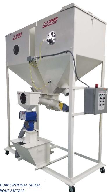
THE VOLUMETRIC BLENDER IN THE PICTURE IS SUPPLIED WITH AN OPTIONAL METAL SEPARATORS FOR THE REMOVAL OF FERROUS AND NON-FERROUS METALS
