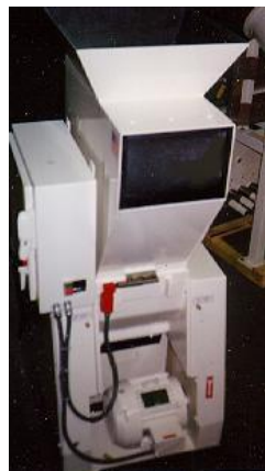
Top feed hopper for conveyor or robot feed
